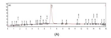
**Figure 1:** HPLC chromatograms of pure standards (A) and *C. roseus* crude aqueous extract alkaloids (B). Stationary phase—reverse-phase Microsorb-MV C<sub>18</sub> column (150 x 4.6 mm); mobile phase-methanol, phosphate buffer, acetonitrile; flow-rate of mobile phase-0.2 ml/min; detection wavelength-254 nm; injection sample volume-20 µl *(continued on next page).*
